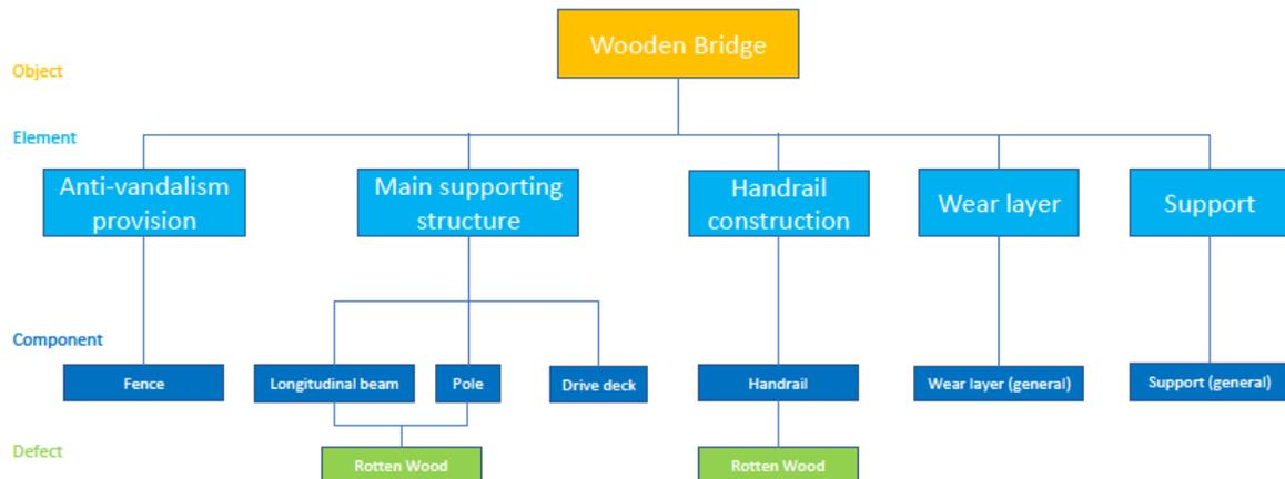
Figure 11 - Schematic Decomposition of Wooden Bridge
