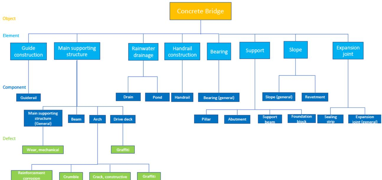
Figure 17 - Schematic Decomposition of Concrete Bridge
